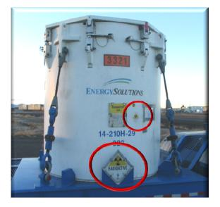
For a Type B cask, it is recommended that the placards be applied to the lower impact limiter to prevent damage to the painted surface on the shielded part of the cask. Pictured is a bulk packaging <640 ft<sup>3</sup> that requires radioactive Yellow-III labels and is utilizing the placarding exception in 49 CFR 172.514(c) because this smaller bulk packaging is labeled.
