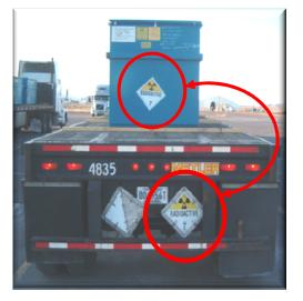
Another option for bulk packagings (<640 ft<sup>3</sup>) is to label each package and include 4 placards on the trailer. Yes, DOT stated that the labeling exception for LSA/SCO exclusive use, domestic, ground and <A<sub>2</sub> quantity in an excepted general design package is just that, an exception. You may still choose to label the package and then placard the vehicle.
